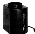
HZ-610MDU 10:1 Motorized zoom lens • C-mount for 1/3" 3-CCD camera • Focal length: 6 mm to 60mm
