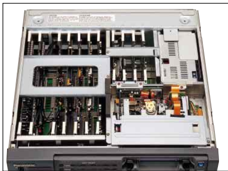
Boards containing LSI chips are easily plugged in or removed. Simply add or exchange boards to expand the interfaces.
