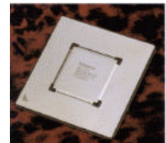
Next-generation digital process ASIC 0.18 \mu m rule
