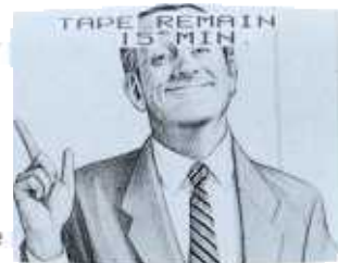
When the above indication appears, the tape remaining time is approximately 15 min.
