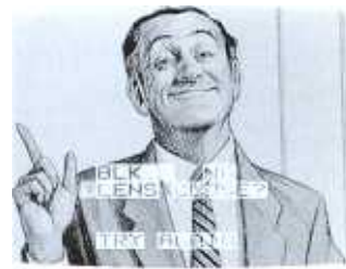
The lens iris is not closed. Check the functions of the lens or the connection of the lens plug.
