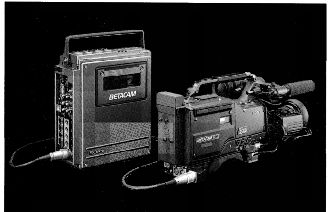
26-pin interface between the BVW-400 with the BKW-402 and the BVW-35 via the CCZ cable
